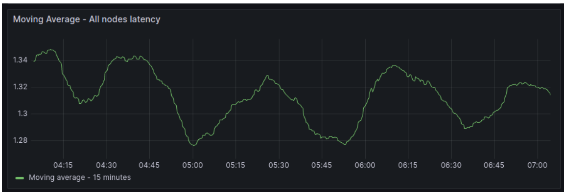
Figure 4.11: eBPF: Moving average of the Round trip over time.
