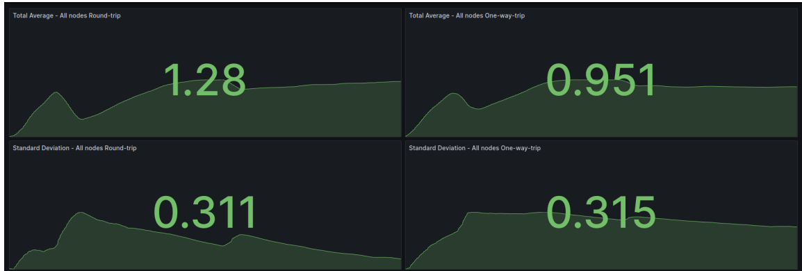
Figure 4.1: iptables: Average and standard deviation gathered from all data points for both Round-trip and One-way-trip.
