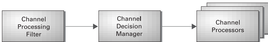
Figure 11.9 A channel-processing filter relies on a channel decision manager to decide whether to switch to/from a secure channel. If a switch is necessary, a channel processor makes the switch.
